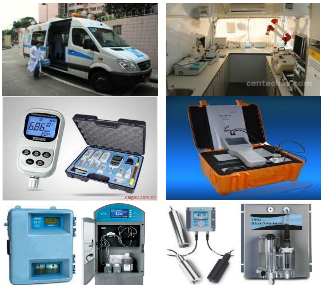
Figure VI.5: Typical Mobile Laboratory, and Portable and Online Water Quality Monitoring Instruments
