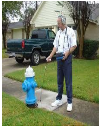
Figures VI.2–VI.3: Acoustic loggers and digital ground microphone for leak detection
