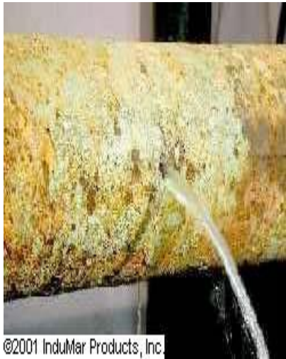
Figure VI.1: Typical water leak due to aged pipe
