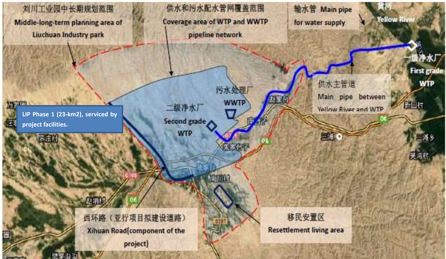
Figure III-2: Layout of the Proposed Infrastructure (in blue: LIP Phase 1, 23-km 2 )
