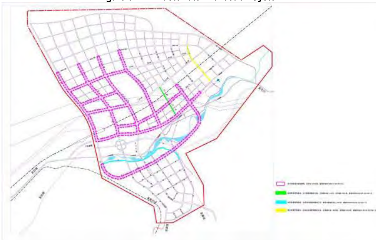
Figure 8: LIP Wastewater Collection System
