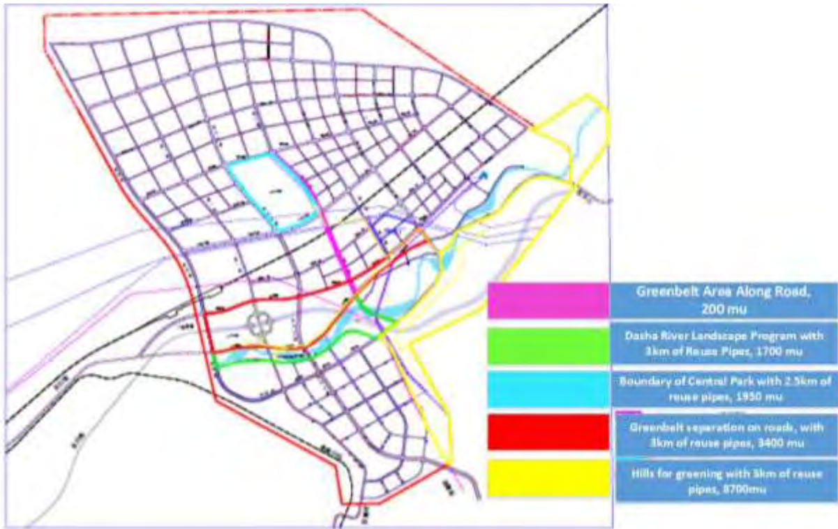
Figure III-8: LIP Treated Wastewater Reuse Piping System for Irrigation. Source: LMC
