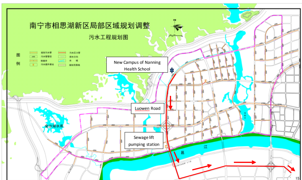
Figure V.2: Sewage Network Plan for Xiangsihu New District of Nanning
