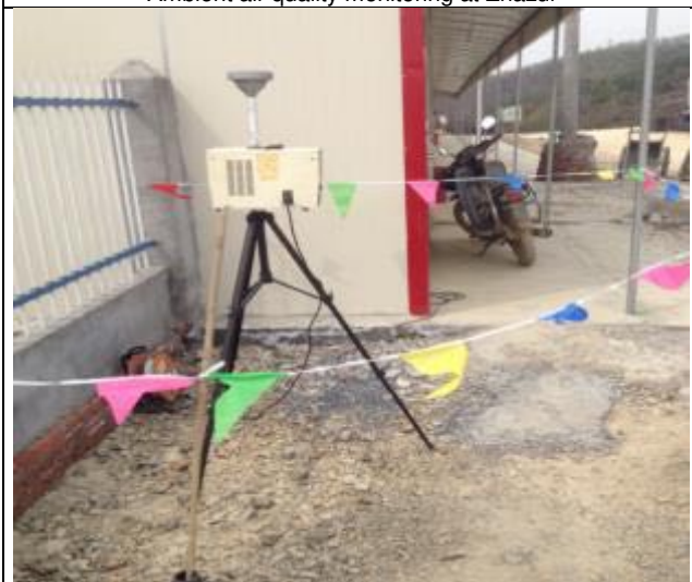
Ambient air quality monitoring at asphalt mixing station
