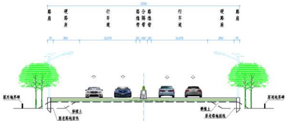
Figure III.11: Typical Cross Section of the Highway
