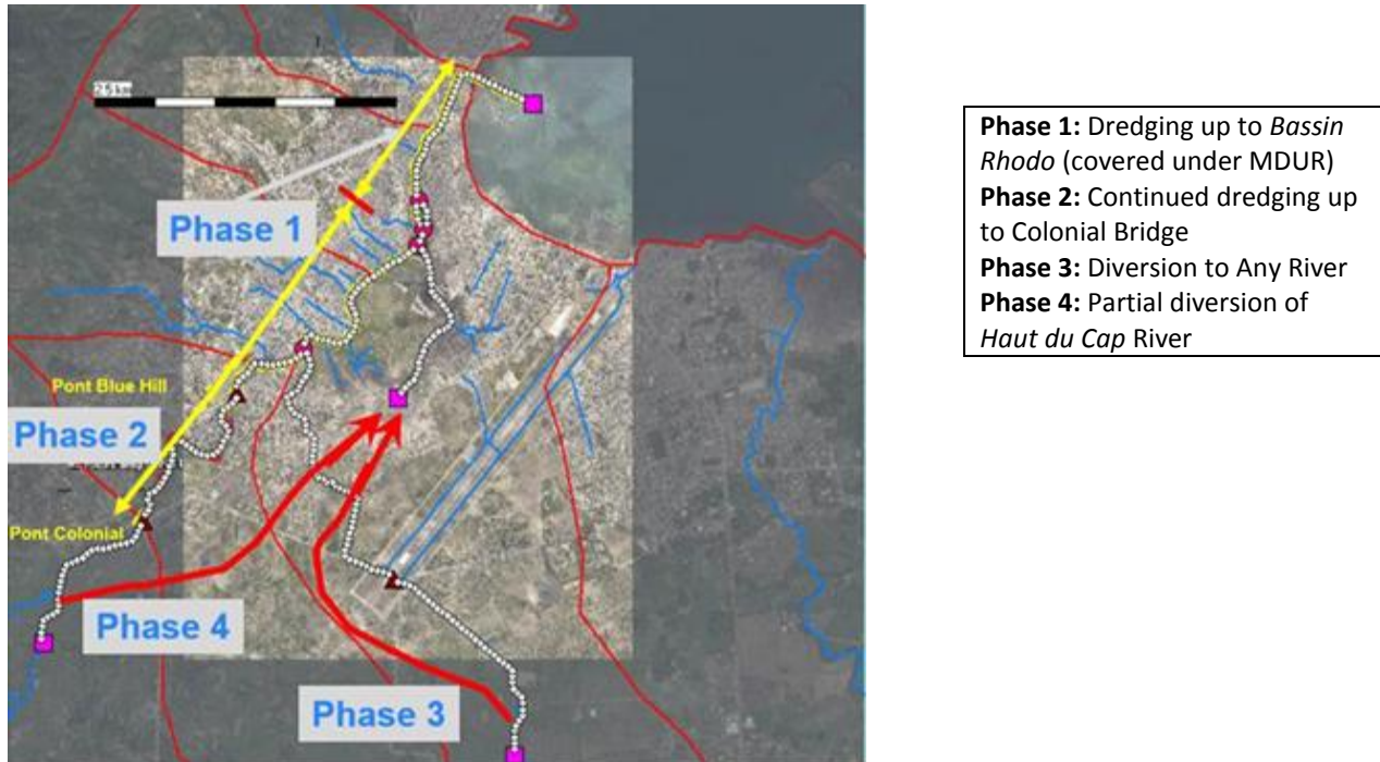
Figure 1: Map of the proposed hydraulic interventions under Component 1 (the first phase will be financed under the MDUR project)
