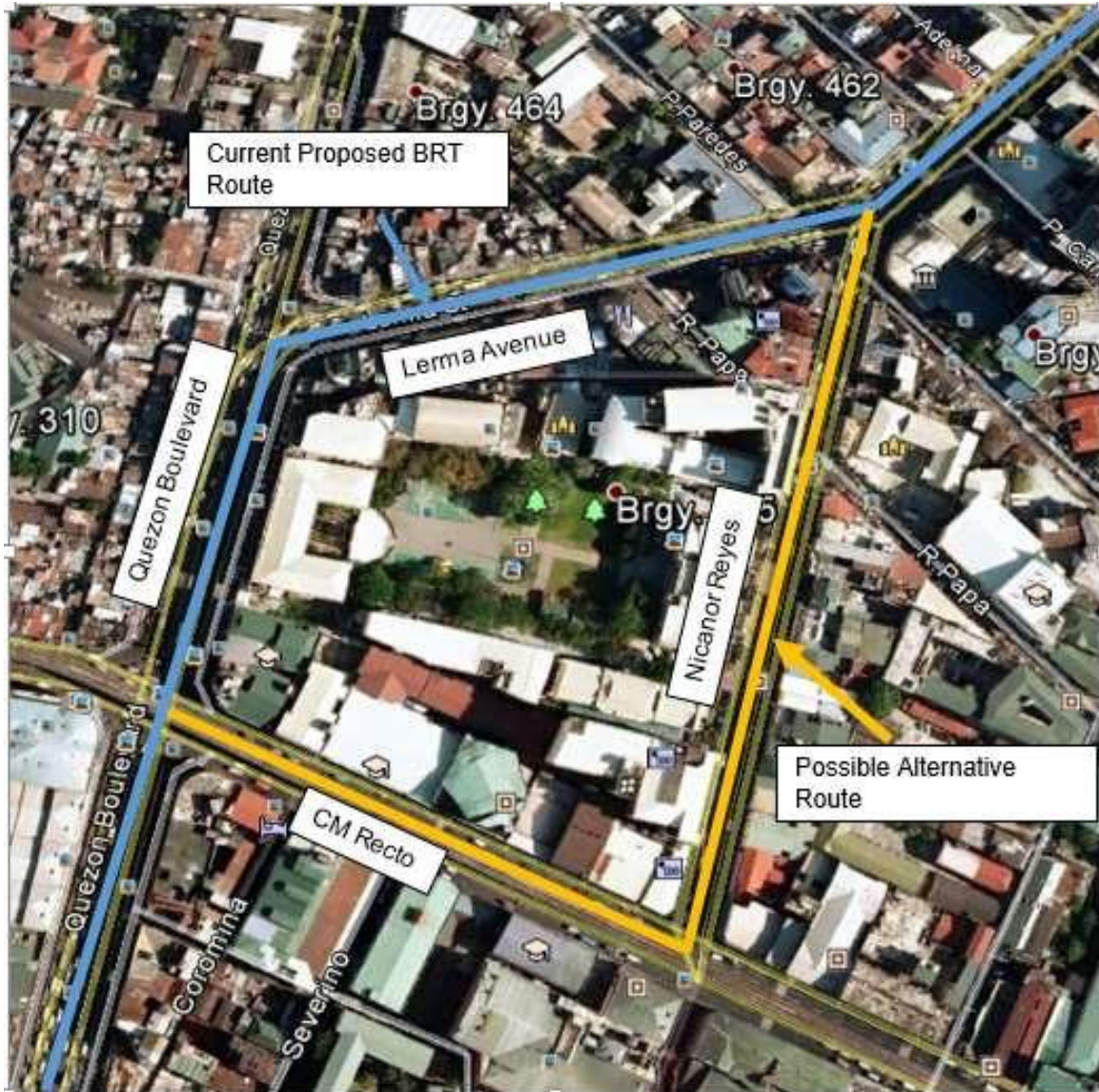
Figure 6.3.2: Alternative BRT Routes via (1) Nicanor Reyes and CM Recto Avenue and (2) Lerma Avenue and Quezon Boulevard
