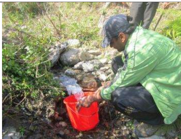
Water discharge measurement at sanohaku
