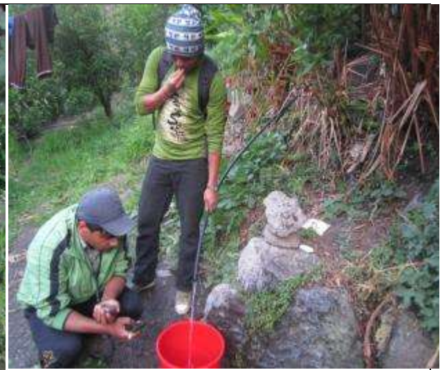
Warmrang mul, measurement the water discharge and Gps point located
