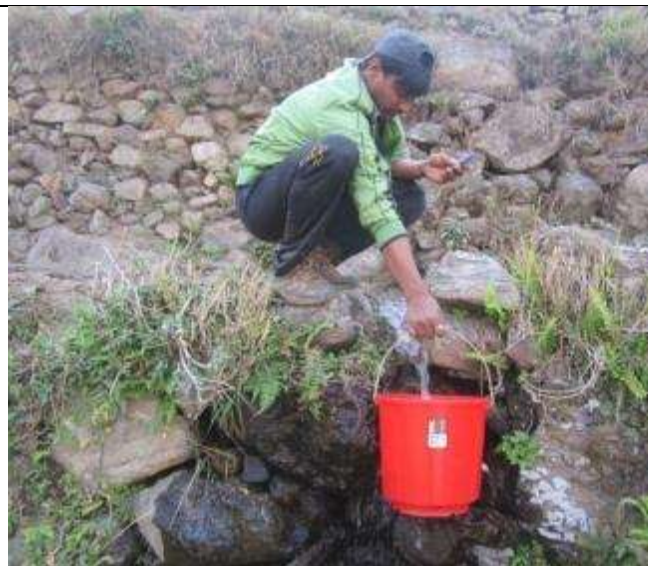
Water discharge measurement at gogane
