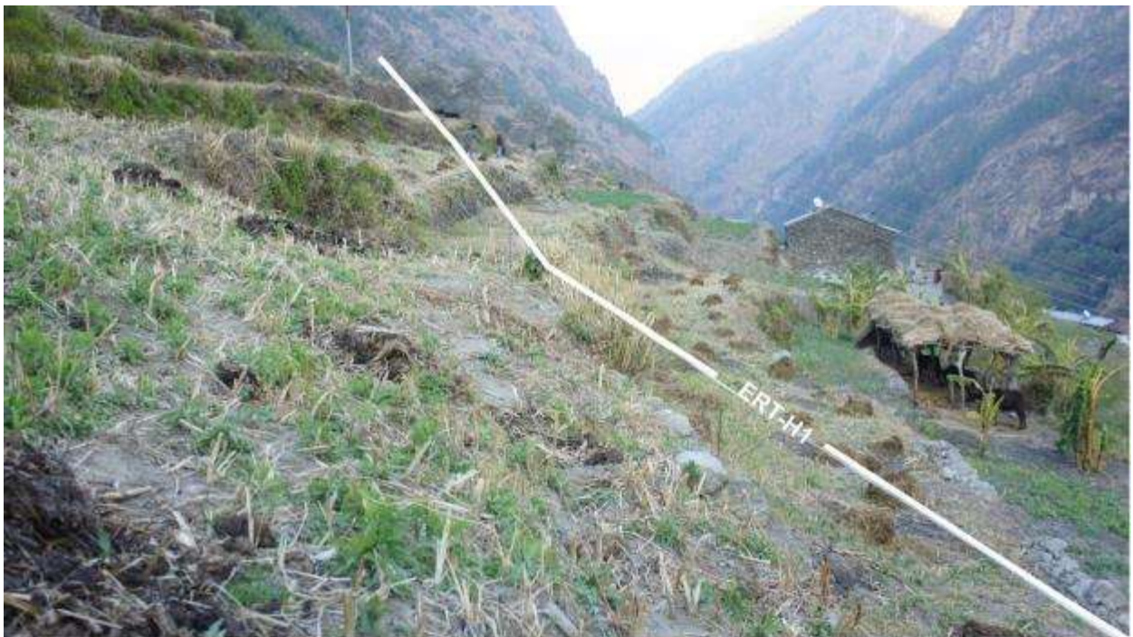
Figure 5-13: Photograph showing the lithology along ERT-H1 (view to the northeast). The white solid line in the figure represents the segment of ERT-H1. A few large boulder are also seen in the figure.
