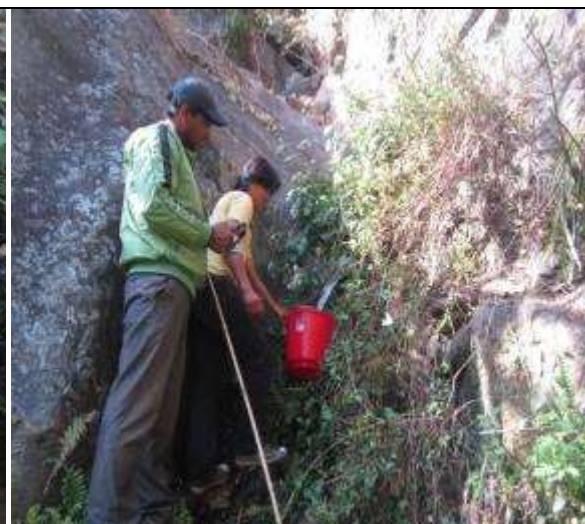
Gumboating spring mul ,measurement the water discharge and Gps located
