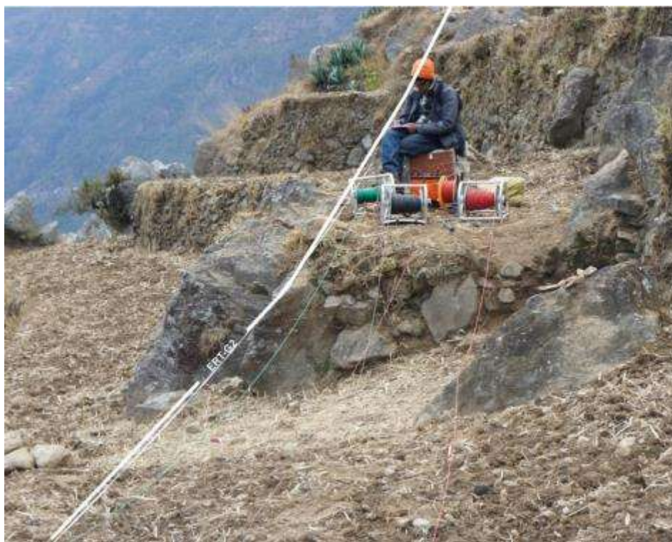
Figure 5-7 Photograph showing the lithology along ERT-G2 (view to the northwest). The white solid line in the figure represents the segment of ERT-G2. A few large boulder are also seen in the figure.
