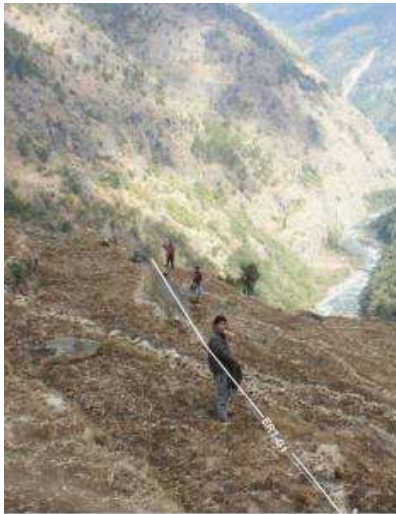
Figure 5-4: Photograph showing the lithology along ERT-G1 (view to the northeast). The white solid line in the figure represents the segment of ERT-G1. A few large boulder are also seen in the figure
