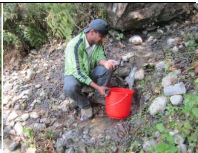
Water discharge measurement and Gps point located
