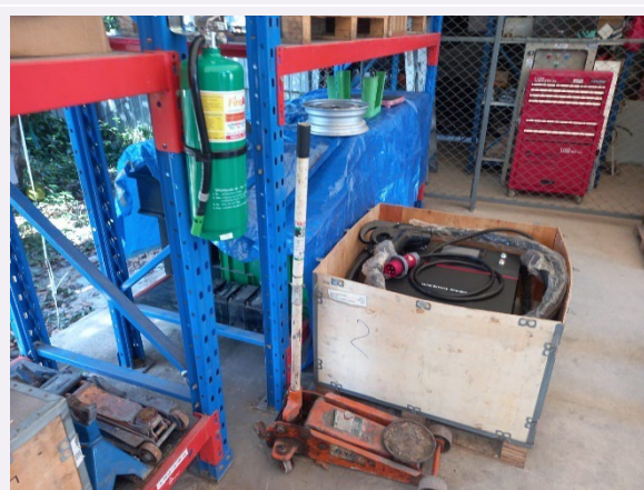
Photo 6: Waste/spent batteries (from the e-tuktuks) stored at the open-air shelving; fire extinguisher provided on the shelving rack
