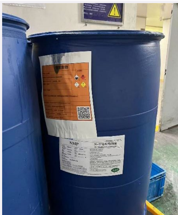
Photo 42: Storage of hazardous waste (waste N-Methyl Pyrrolidone) in the hazardous waste storage room
