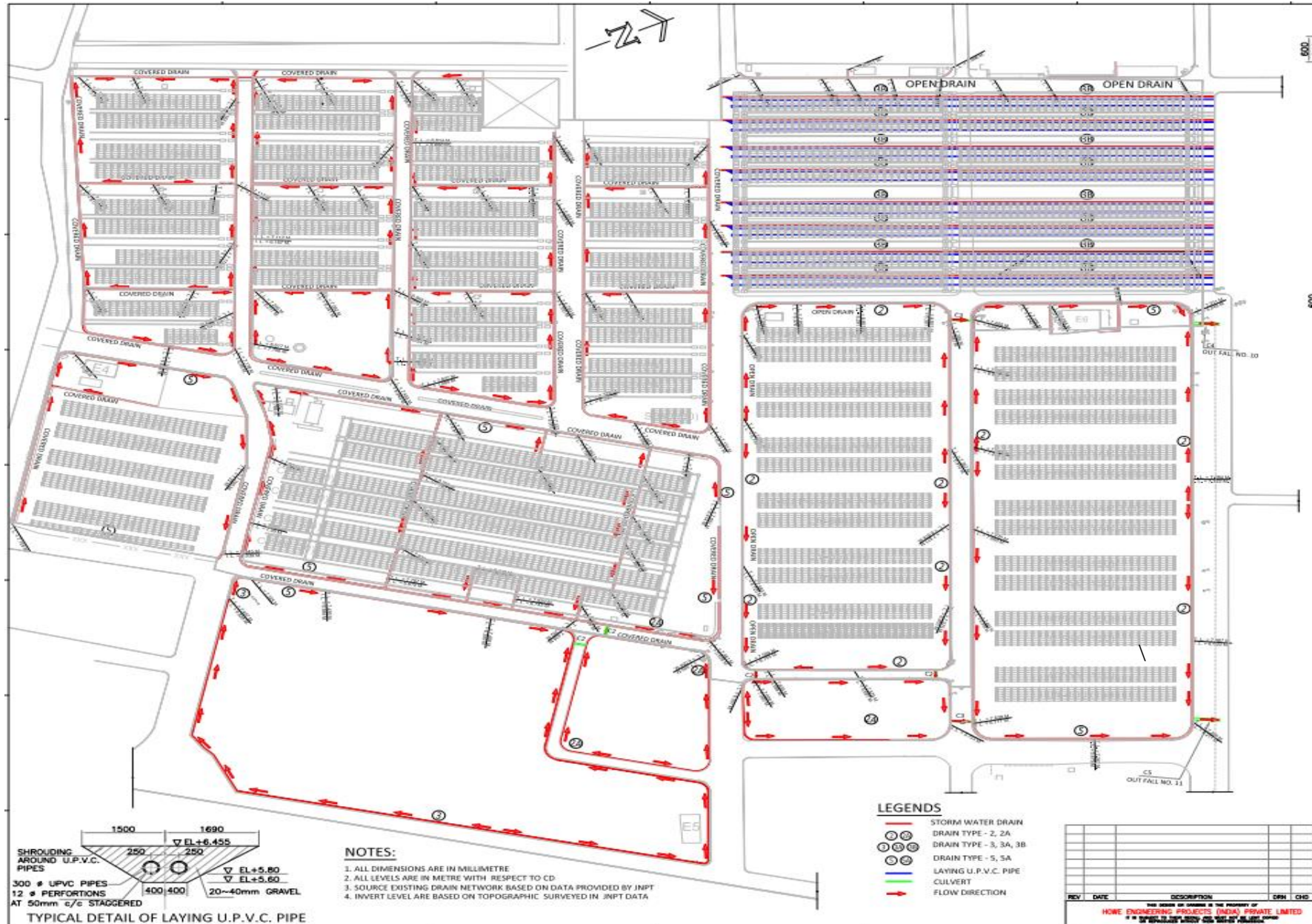
Figure 2-9: Existing Stormwater Drainage at JNPCT
