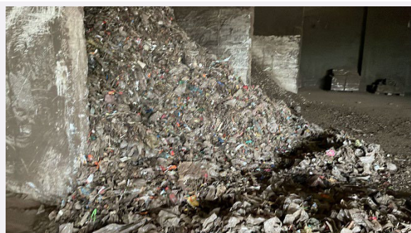
Photo 51: Process of final product refinement at compost plants 1 to 3. Plastic rejects directed to the WtE.
