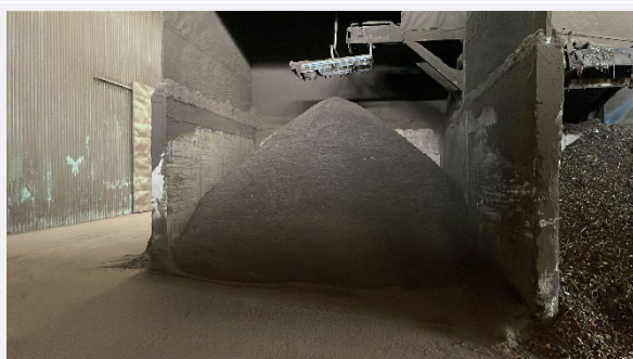
Photo 54: Process of final product refinement at compost plants 1 to 3 with refined humus.
