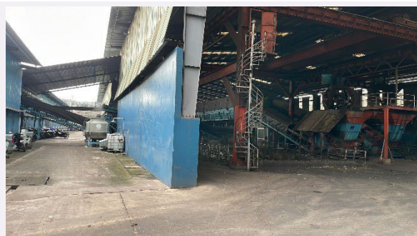
Photo 49: Raw waste visible in the right side of the photo is passed through a trommel screen and fractions are conveyed to the left which is the fermentation plant.
