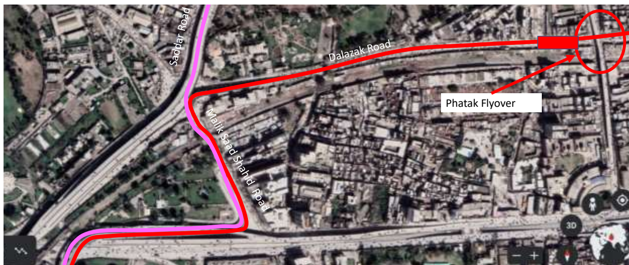
Figure 4. The Dalazak Road BRT corridor must serve the existing direct service BRT Routes 3 and 4 (pink) and new Dalazak Road BRT services (red). The elevated structure will also need to be constructed for grade separation at the Phatak Flyover.
