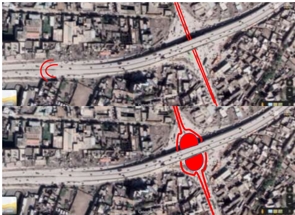
Figure 10. Peshawar Ring Road and Kohat Rd. Interchange shown with two possible BRT alternatives on Kohat Rd.
