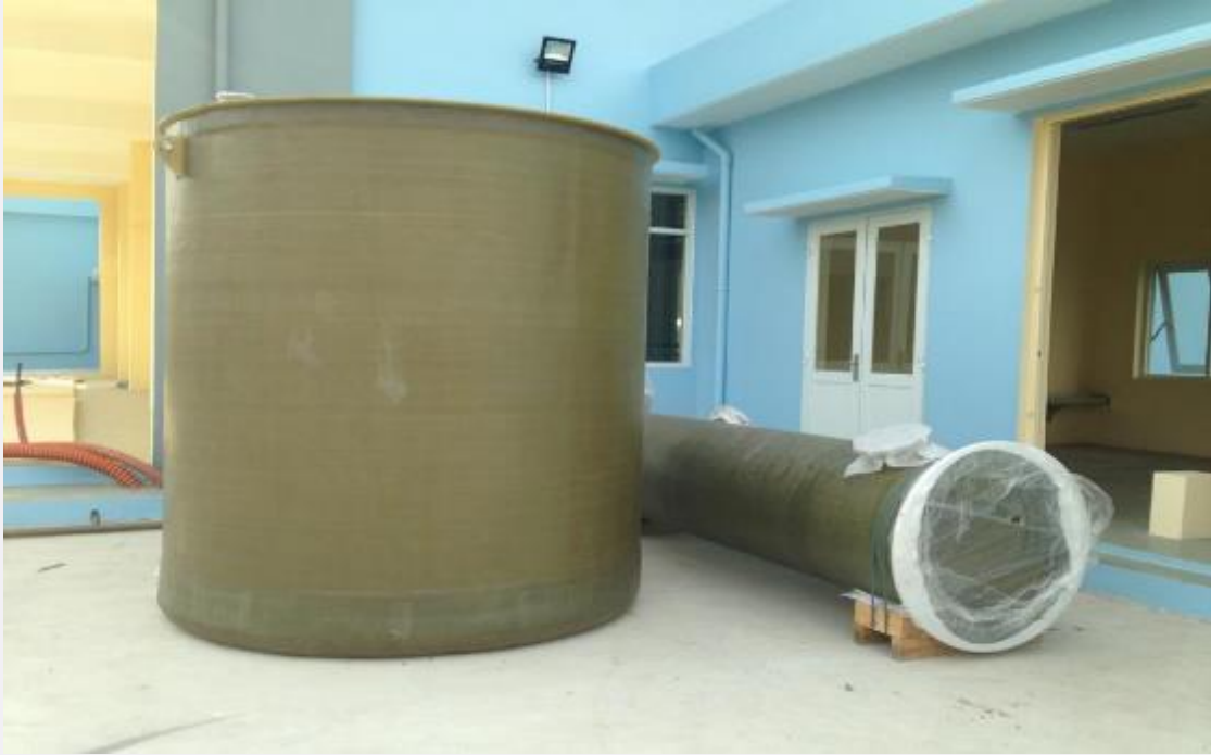
Photo 11: A neutralization tower for the new chlorine house at the Intake Station
