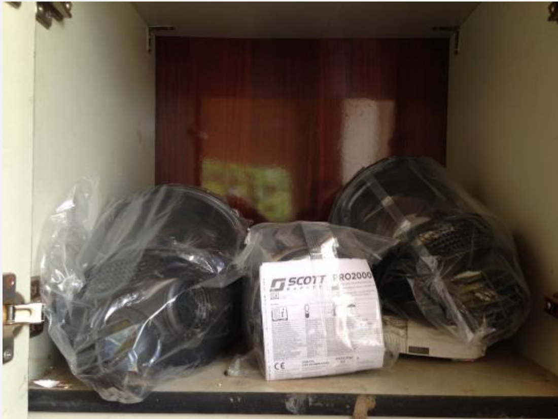
Photo 13: Respirators provided inside the existing chlorine gas storage house at the Intake Station
