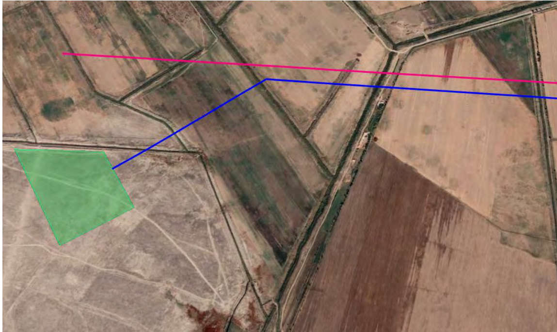
The existing 110kV transmission line is figured in light red The new 220kV transmission line is figured in blue
