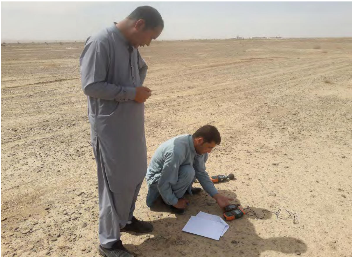
Figure 6. Monitoring of Sound Level.
