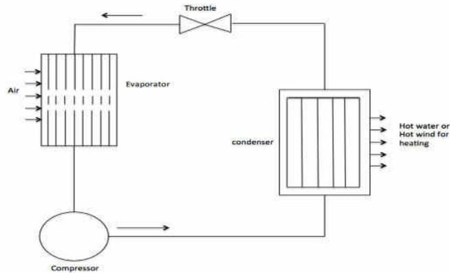
**Figure III-5:** Diagram of Air Source Heat Pump
