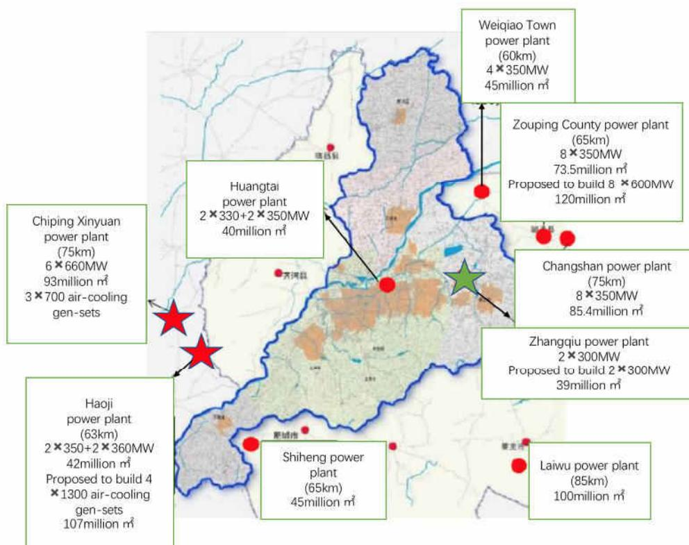
**Figure III-3: Waste Heat Sources around Jinan**
