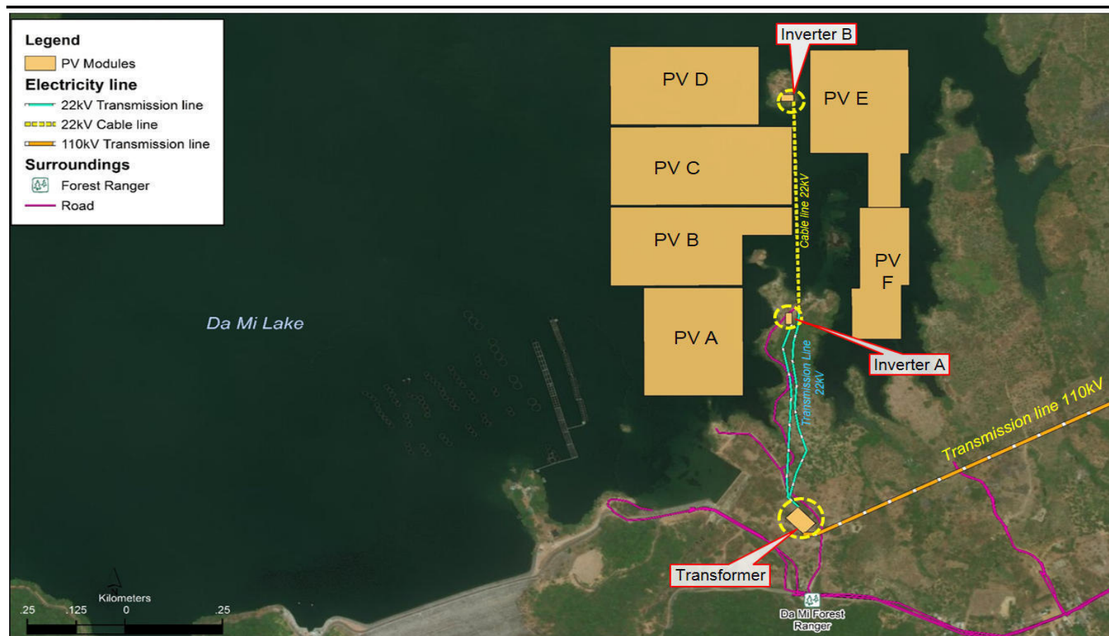
Figure 5. The Location of PV Module on the Surface of the Da Mi Hydropower Reservoir
