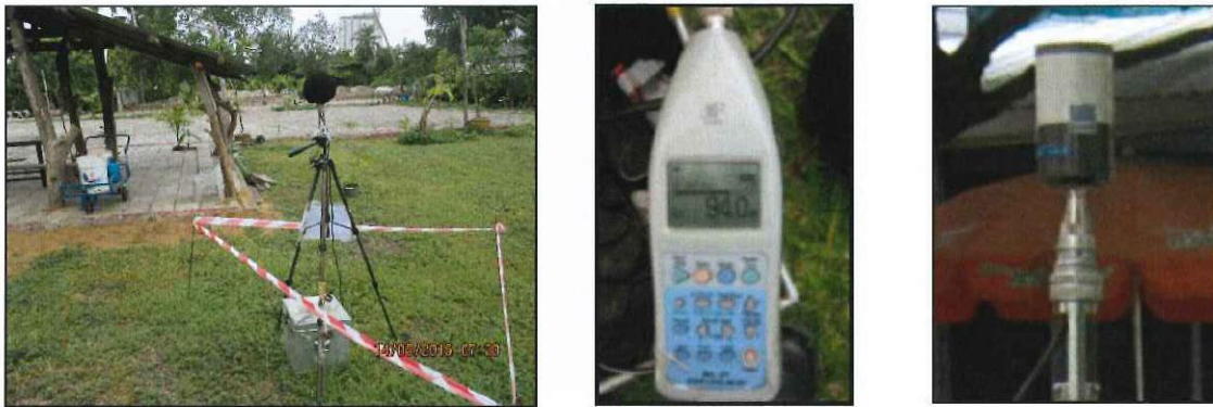
Figure 2-9: Monitoring the sound level by using Integrated Sound Level Meter and Acoustic Calibrator produced sound wave with frequency 100 Hz 94.0 dB.
