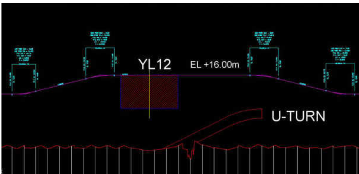
Figure 2.1.3 – 13 Plan and Cross Section of Guide Way at Khokwat Canal U-turn Bridge
