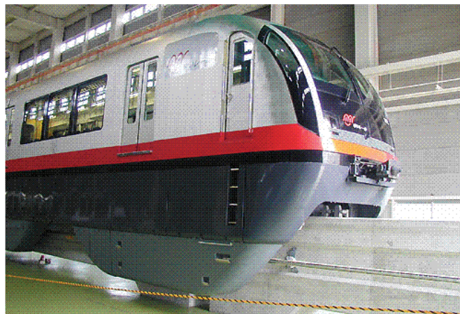
Figure 5.1-9 Straddle Monorail Type, the Train Straddles the Track
