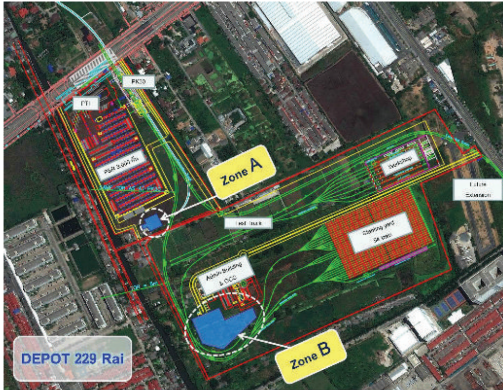
Figure 5.1-1 Retention Ponds in the Depot and Park & Ride Building Area, Rom Klao Intersection
