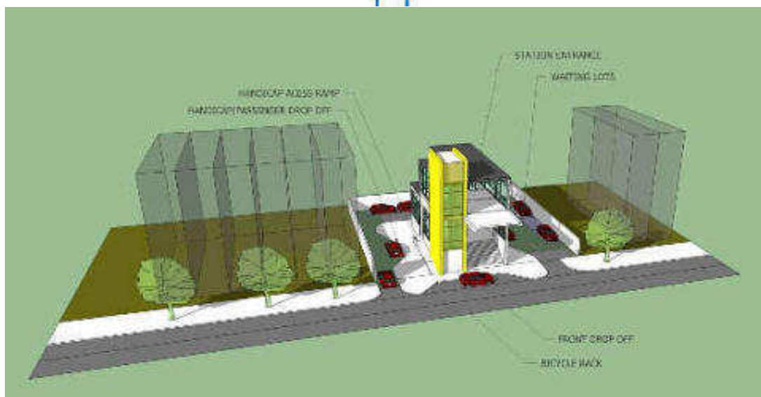
Figure 3.6.2 - 3 Example of passengers Drop off at MRT station
