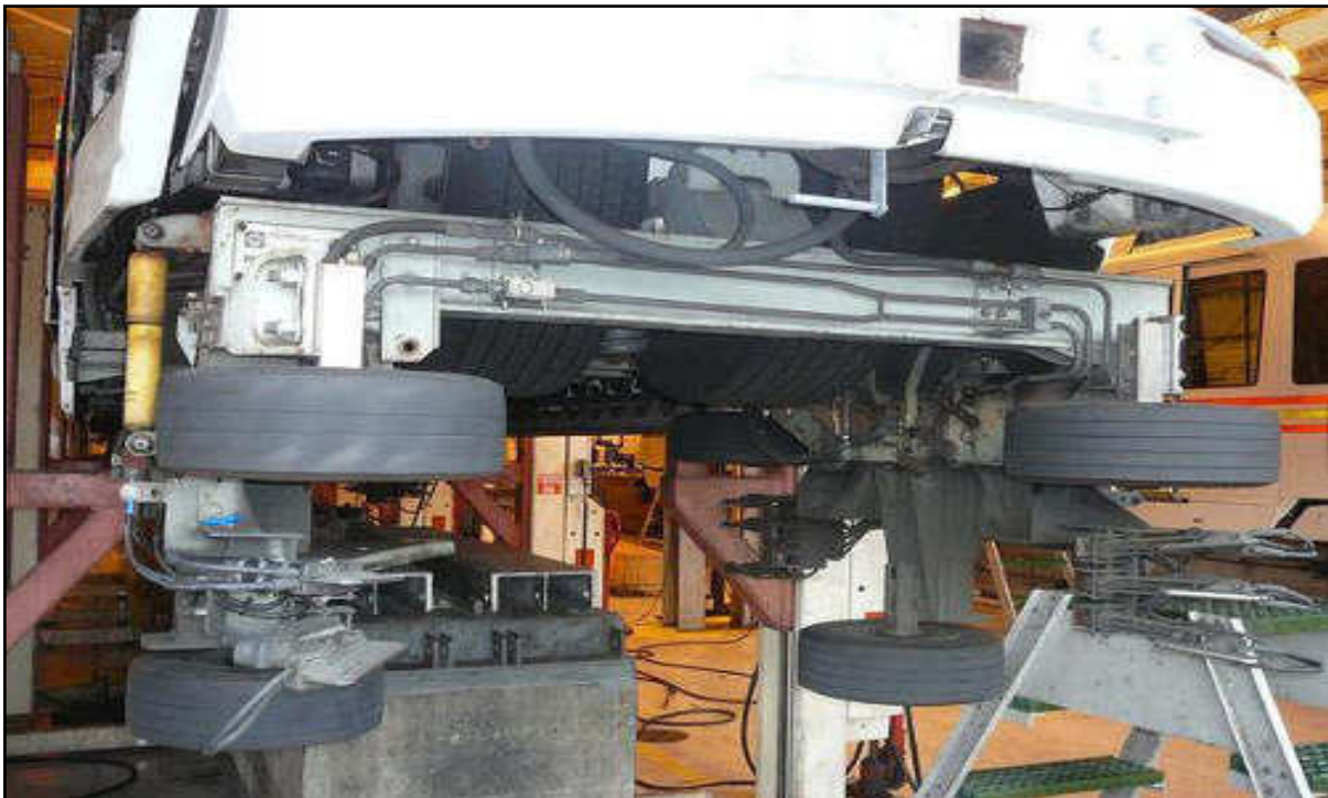
Figure 3.9.3 - 7 The Wheel Diagnostic and Tyre Replacement tools
