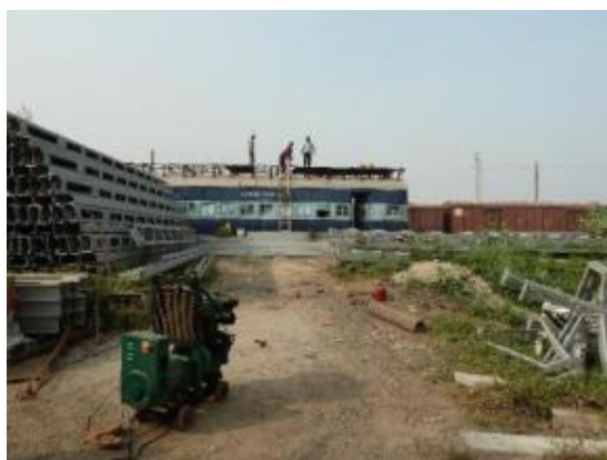
Modified wagon used for erecting overhead lines
