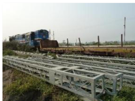
Flat wagon used for transporting the poles
