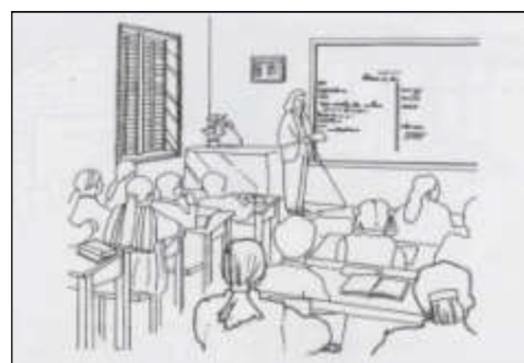
A louvered window could provide glare-free light at the front of classroom
