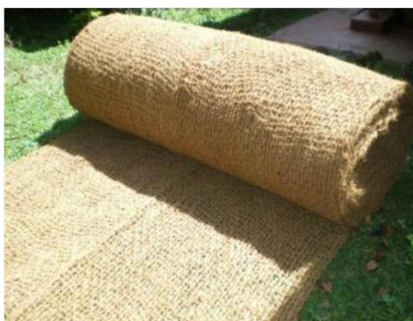
Figure III-28: Coconut fiber (CF) net for slop protection
