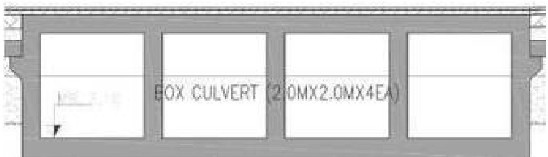
Figure 1-2: Box culverts under the access road with invert level 3.1 m from revised design drawings
