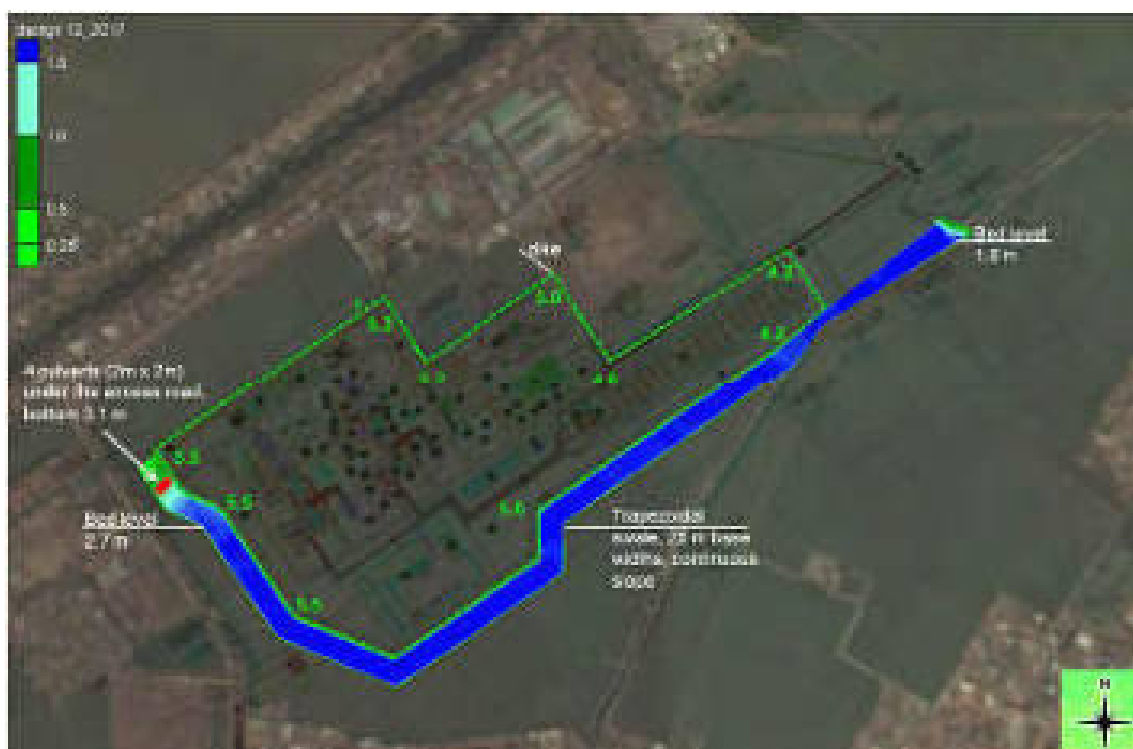
Figure 1-4: Flood flow path in December 2017 layout (swale, polygon colored by depth below current ground) along the revised green flood dike with proposed dike levels
