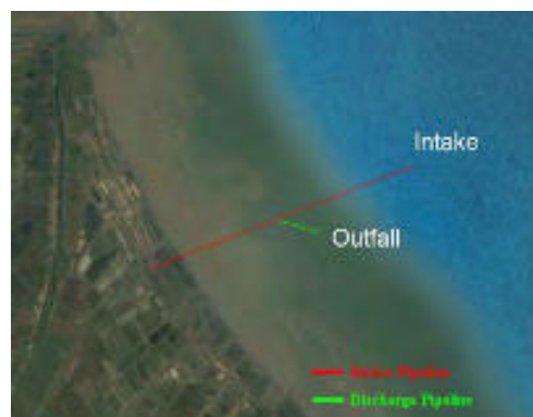
Figure 6.10. Intake and outfall configuration of Jawa 1 CCGT power plant
