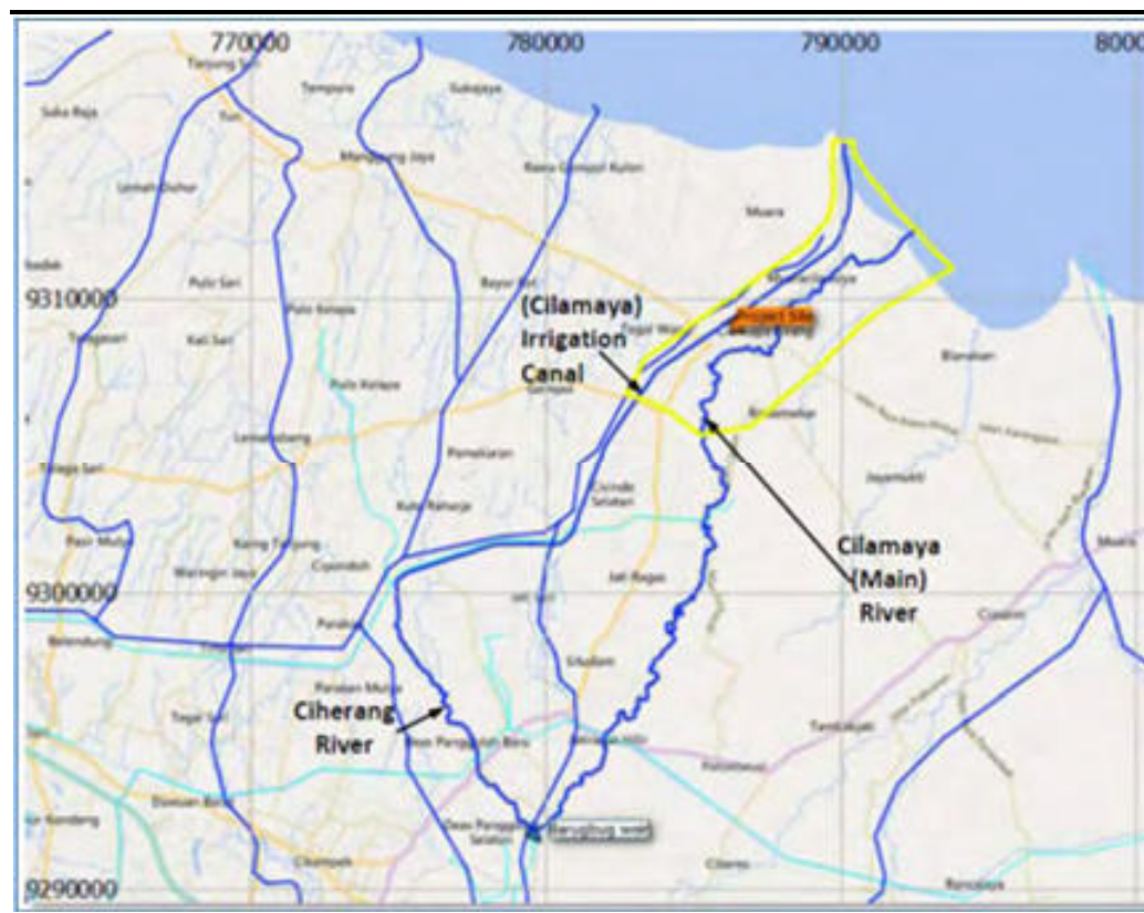
Figure 1.1 Project Site with River and Canal Network (blue) and Main Flood Flow Paths labelled, Barugbug weir and the Preliminary Hydraulic Model Domain (yellow)
