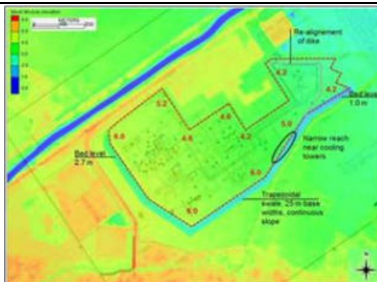
Figure 6.2 Proposed Flood Flow Path (Swale) Along the Revised Flood Dike (Red Line) with Dike Levels, Suggested Re-Alignment at the Downstream Dike Reach (Grey) and Ground Elevations (Coloured)
