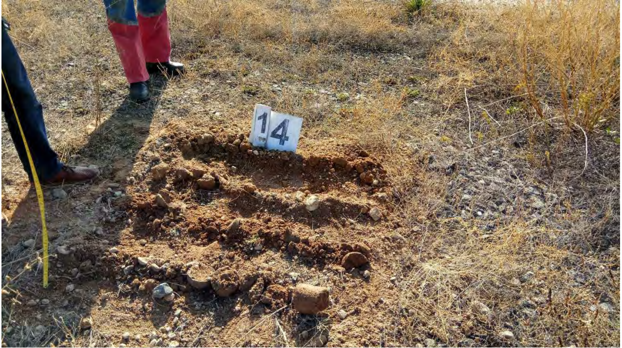
Foto 10: Drilling core from borehole 14 ready to take sample.
