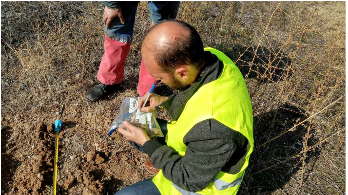
Foto 11 : Taking soil sample from borehole 14 in plastic bag
