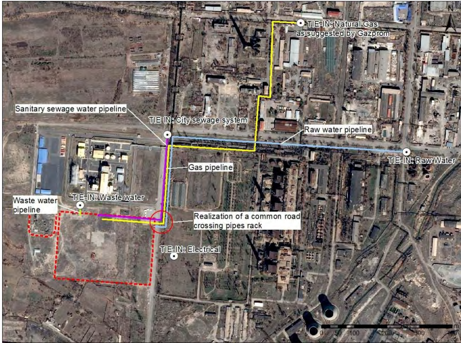
Figure 3-3: Overview plan showing the new interconnections of YCCPP-2
