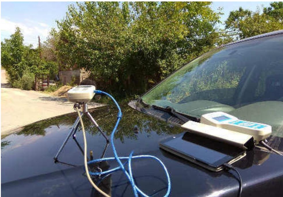
Figure 5. Measurement process at point Noise 5
