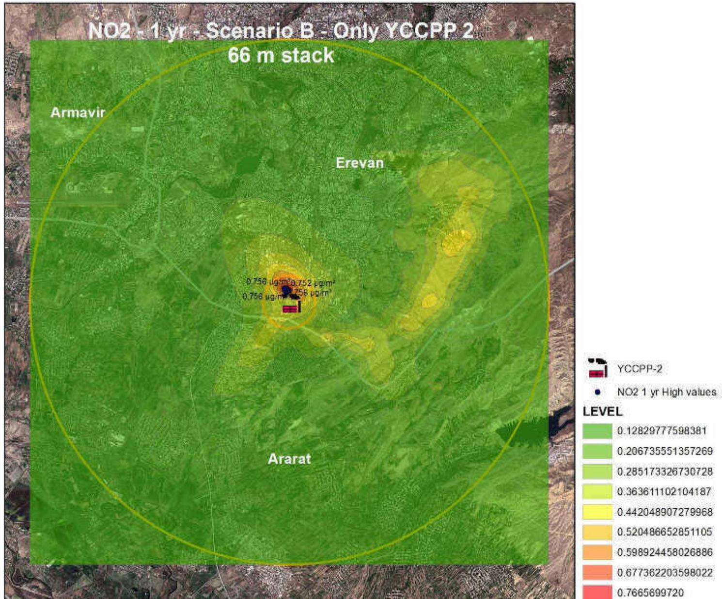
Figure 5-7: Maximum simulated 1 yr NO<sub>2</sub> GLC - Scenario B - YCCPP 2 only
