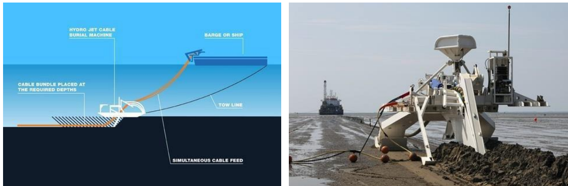
Figure 3.4: Example of Submarine Cable Ploughs
