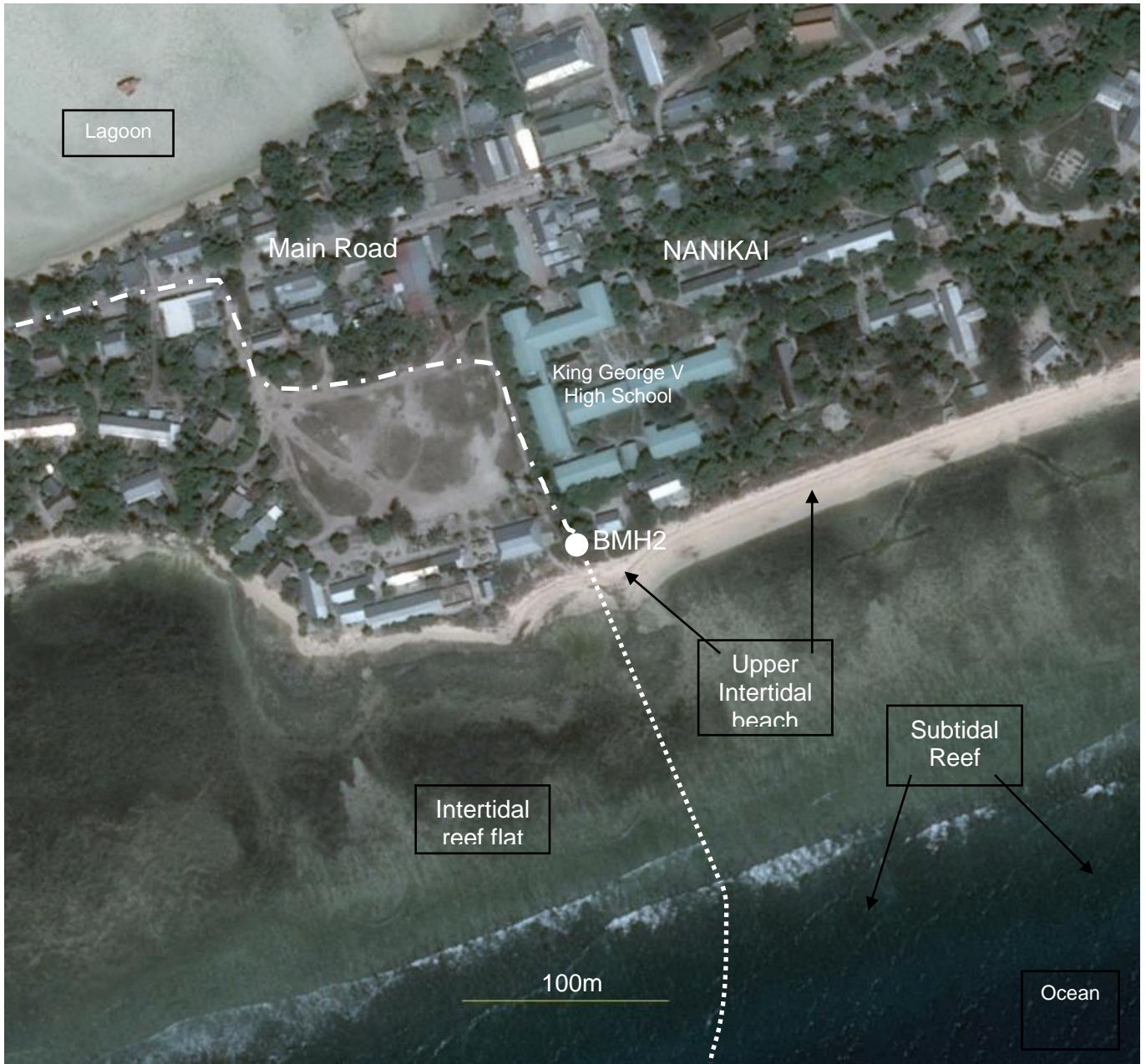
Figure 5e: Potential cable alignments for BMH2 (white dashed lines) in Kiribati
