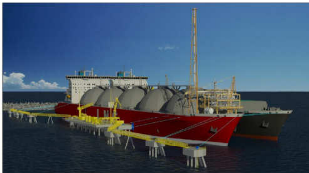
Schematic diagram of FSRU (on Right) and LNGC at Single Berth Jetty
