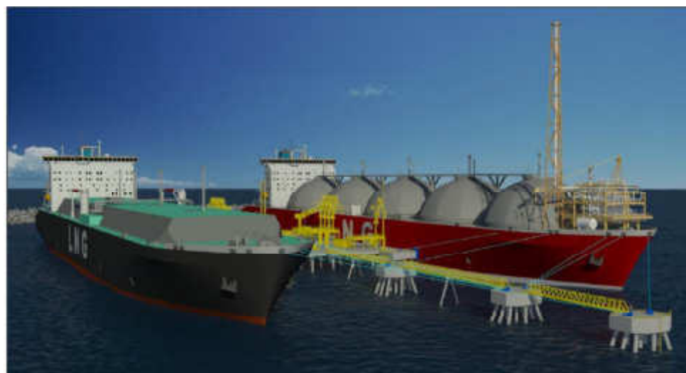
Schematic diagram of FSRU (on Left) and LNGC at Dual Berth Jetty
