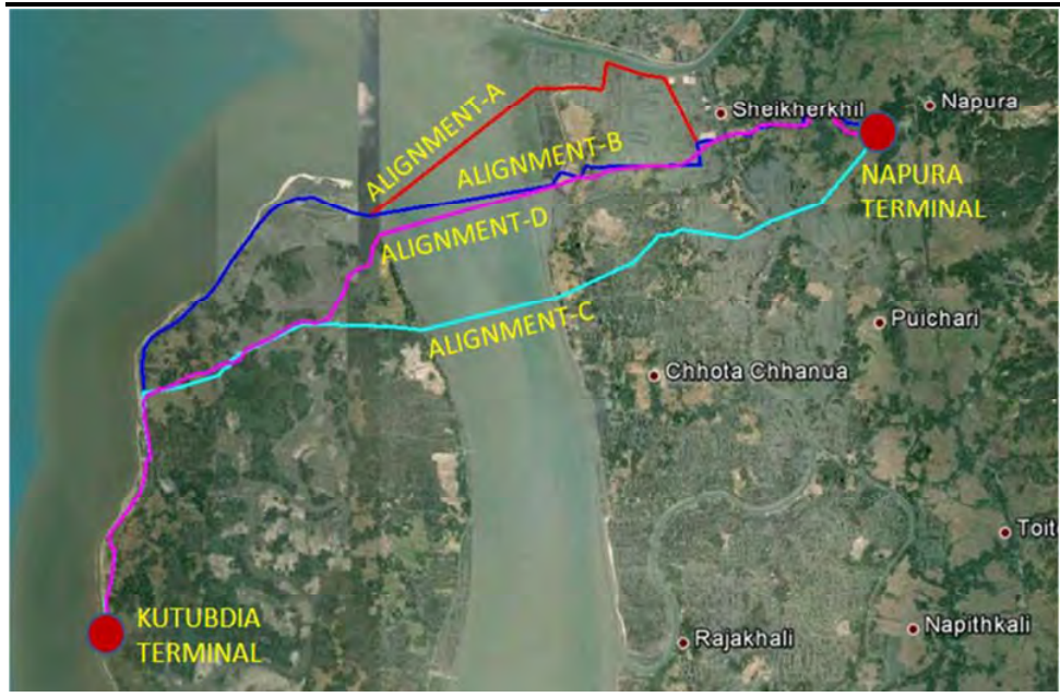
Figure 1.1 Reconnaissance Survey based Four Alternative Pipeline Routes
