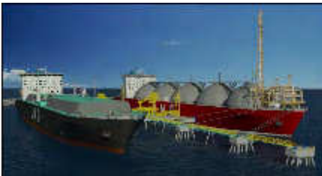
Schematic diagram of FSU (on Right) and LNGC at Dual Berth Jetty
