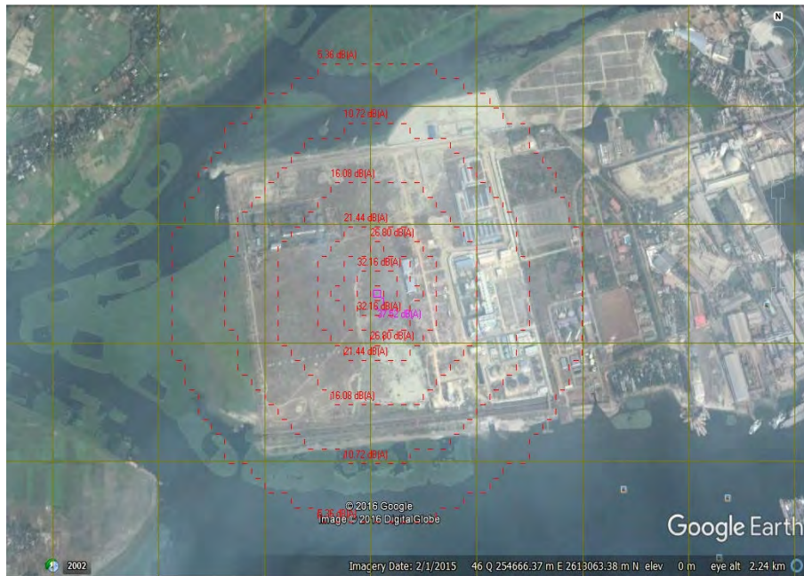
Fig 6.4: Plot of output noise power level in dBA vs Radius in meter
