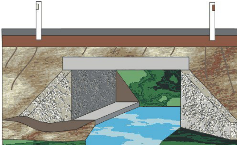
Figure 10-2 Faunal underpass in open bottom culvert
