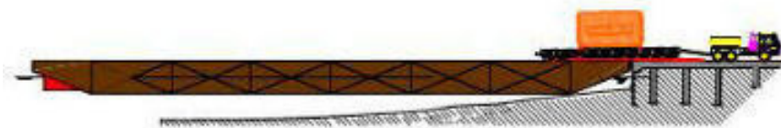
3. Discharging heavy lift cargo from barge by roll off system
