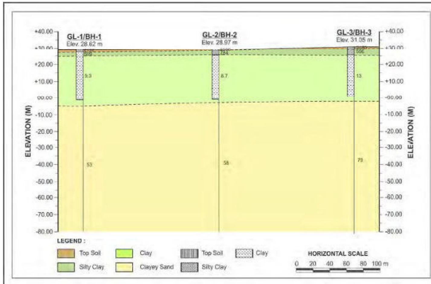
Geological Section Based on Interpretation of Geoelectric and Drilling Result (Log Drill)
