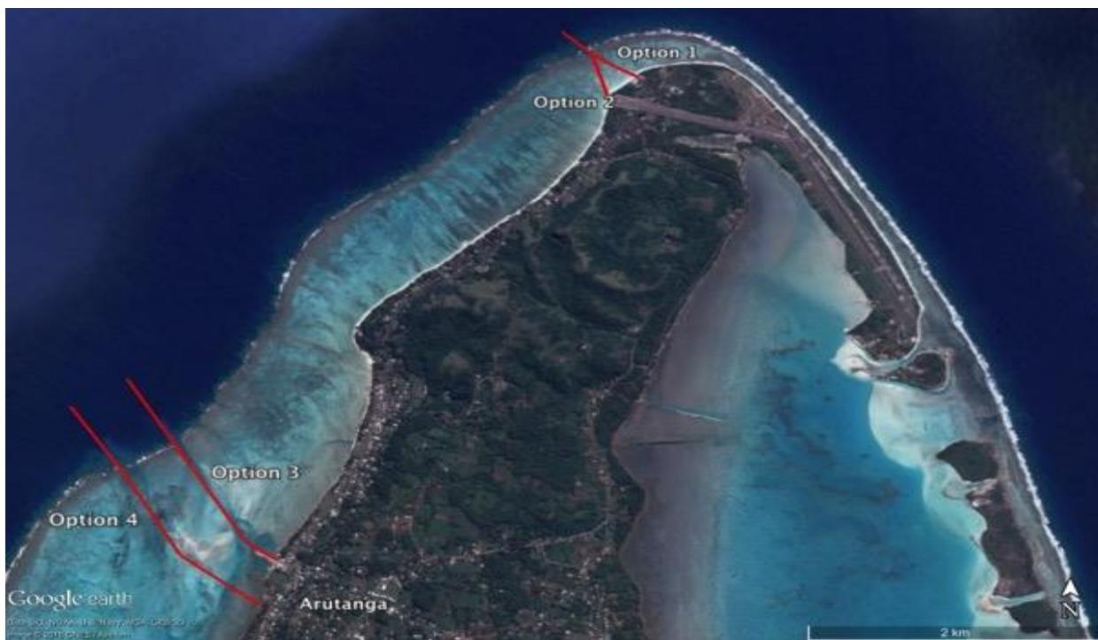
Figure A1.2: The locations of the four cable alignment options sites for Aitutaki
