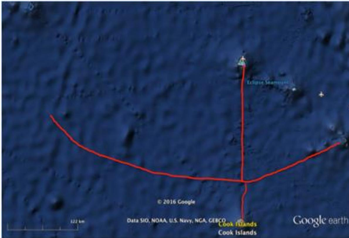
48. **Rarotonga Cable Landing Arrangement and Cable landing station.** Figure 3.3 shows the two indicative marine cable route alignments identified during a previous technical study (No. 1 and 2) and a third identified by the safeguards team in the Rutaki area of Rarotonga's southeast coast. A brief route description follows:
