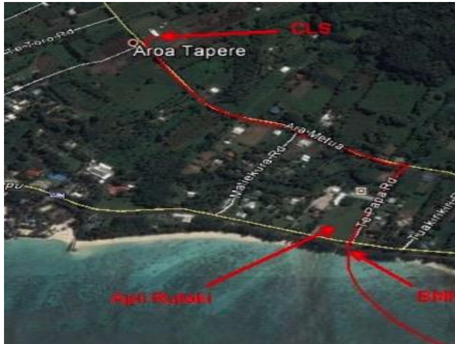
Figure 2. Proposed Rarotonga Cable Landing point, Cable landing Station and Cable Route
