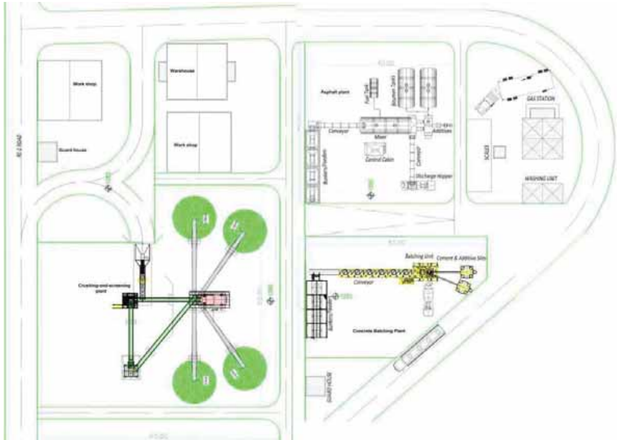
Figure 4.7.2.1. Scheme of Nenskra dam construction site
