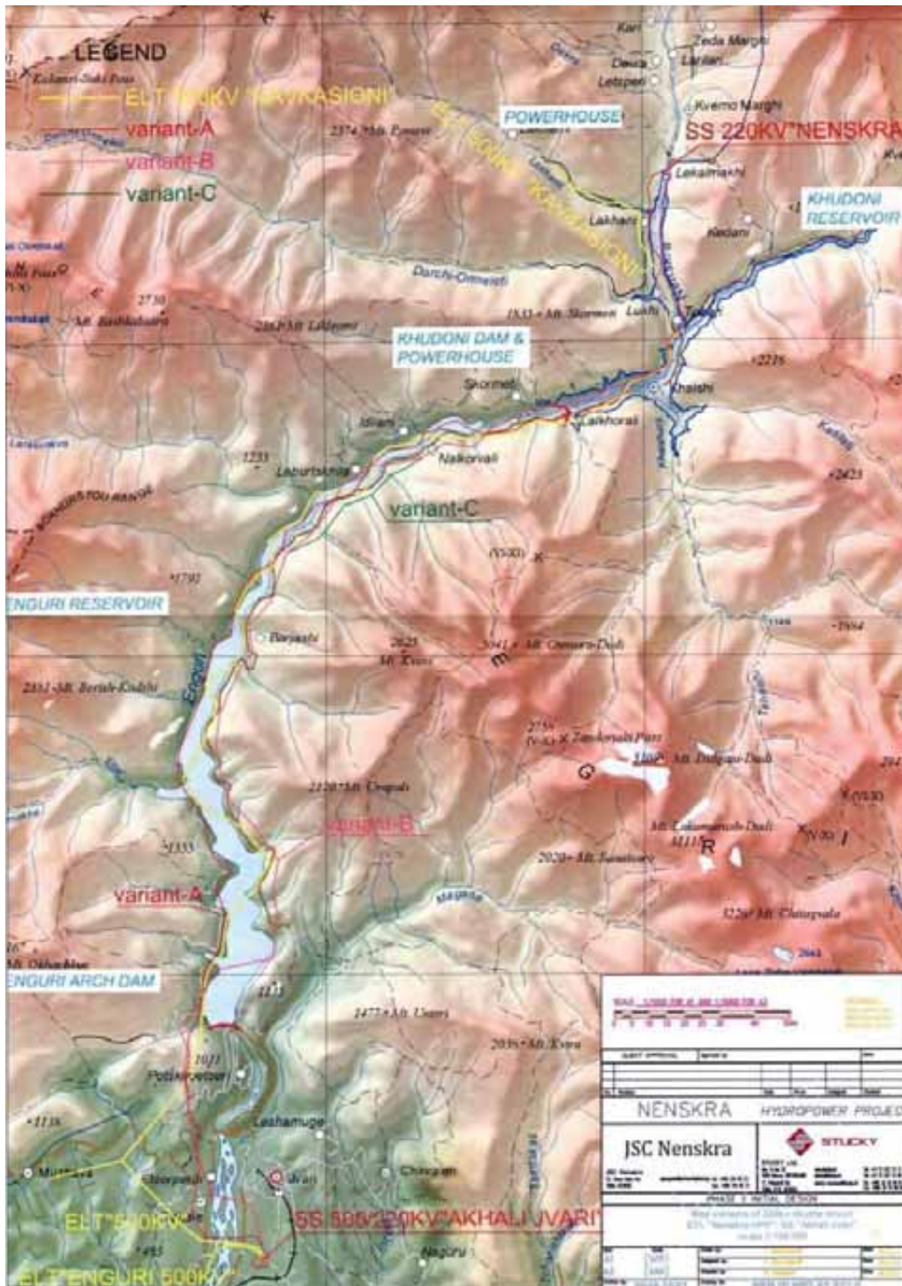
Figure 4.6.1. Scheme of alternatives of transmission lines
