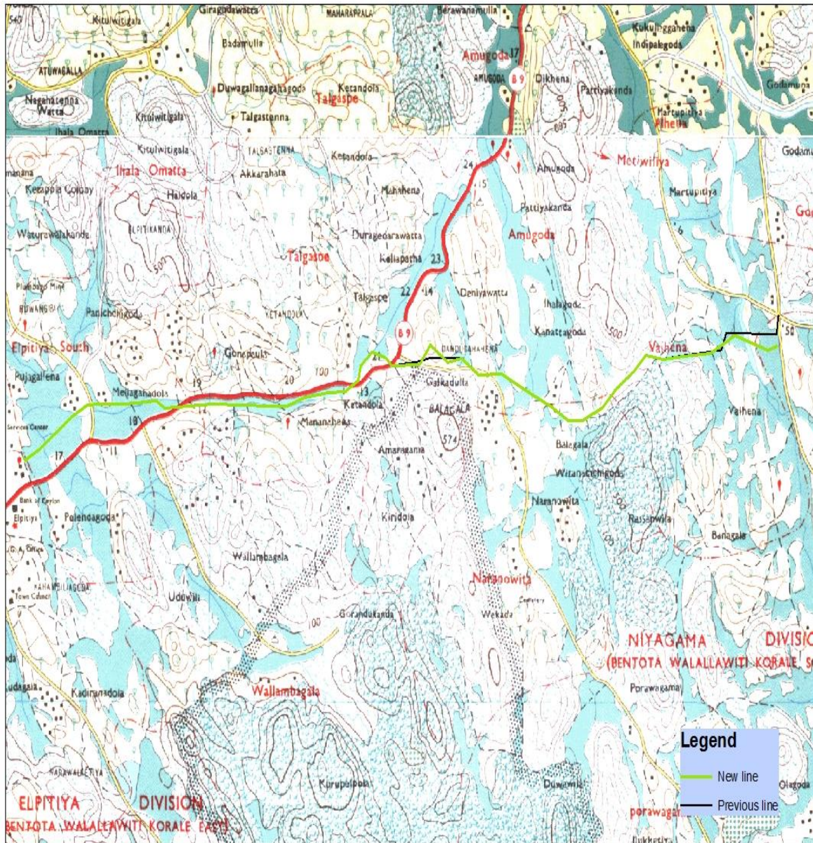
Figure 8: Elpitiya- Mattaka 33 kV line- 11 km
