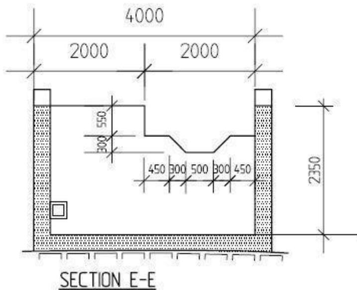
Figure 5 The outlet from fish ladder pool no 3 to no 8 has a notch designed to give good hydraulic conditions with flow up to  $1\text{m}^3/\text{s}$ . This notch is alternating right and left as moving upstream.
