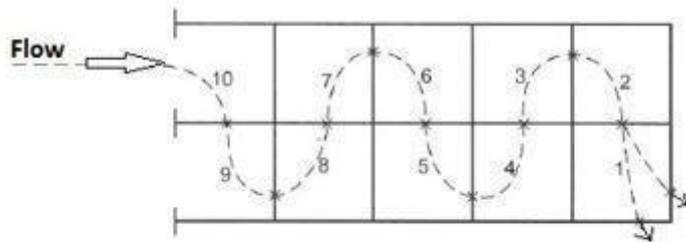
*Figure 8. Examples of compact design of fish ladders.*
