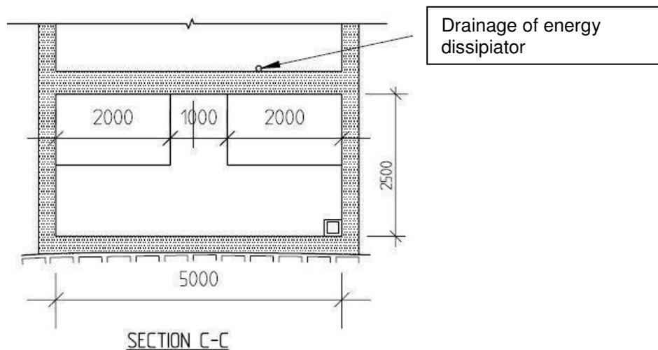
Fig. 3 Outlet from pool no 2 have 2 overflow notches.
