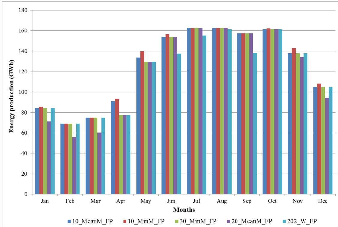
Figure 10.1 Energy production under different EFlows scenarios
