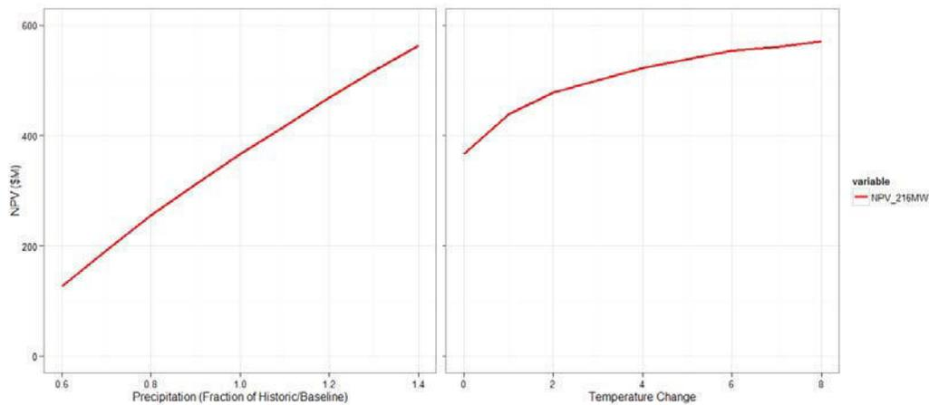
Figure 21 Range of possible economic performance of UT-1 hydropower plant under climate change.
