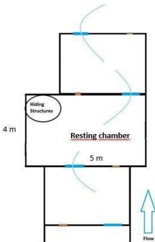
*Figure 7 Resting chamber or resting pool is bigger than the normal fish ladder pools and is equipped with hiding structures at the bottom level in the calm part of the pool.*
