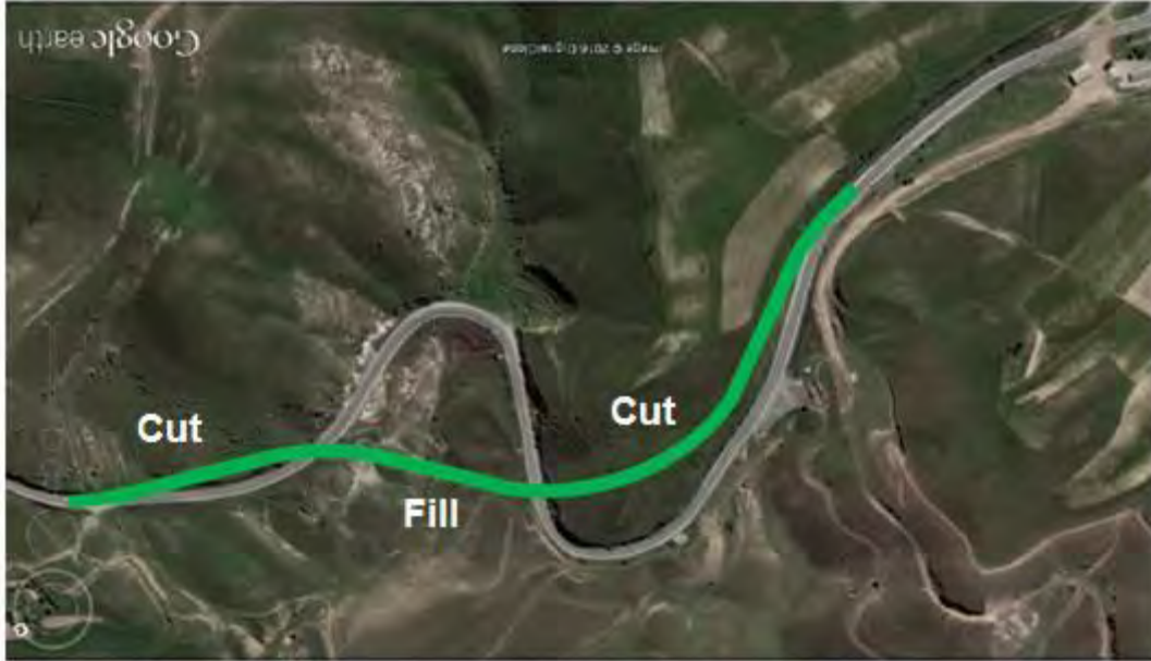
Fig. 3: Chosen alignment mountain section
