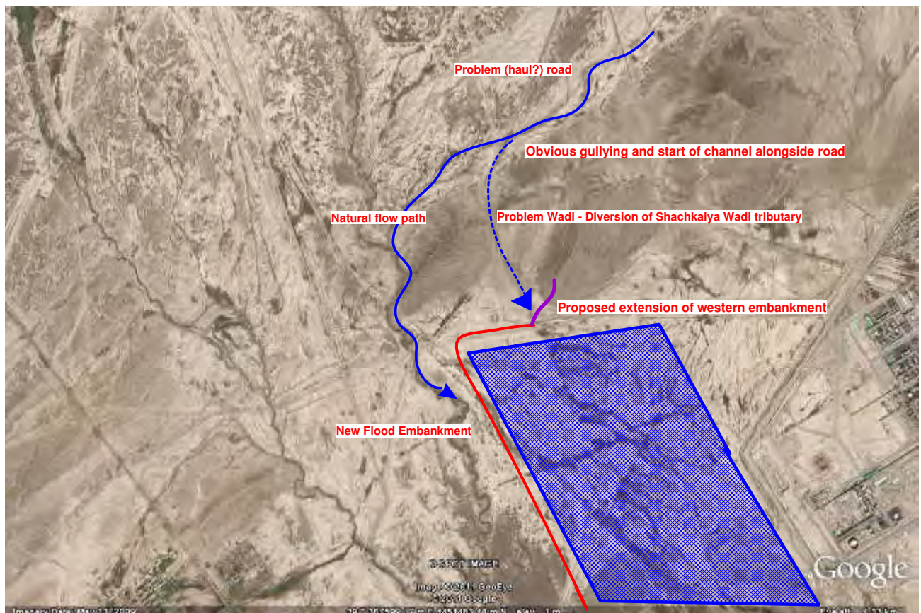
Figure 3.1 Diversion of Wadi by Haul Road North of SD2 Infrastructure area
