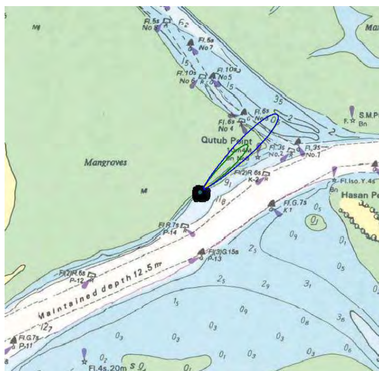
Figure 10: Rupture of transfer hose, with failure of ESD. Flash fire cloud footprintSW Monsoon / Day-time conditions, SW wind Blue: 1/2 LFL; Green: LFL; Yellow: UFL
