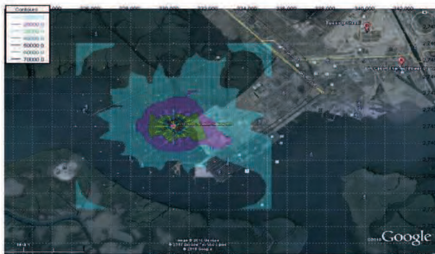
Figure 3: Color average 24-hourly contour map for vapor emission scenario
