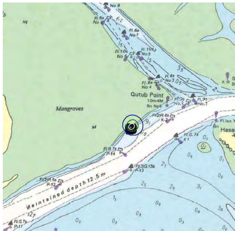
Figure 9 : Rupture of transfer hose, with failure of ESD. Pool fire radiation ellipse SW Monsoon / Day-time conditions, SW wind Blue: 4 kW/m 2 ; Green: 12.5 kW/m 2 ; Yellow: 37.5 kW/m 2
