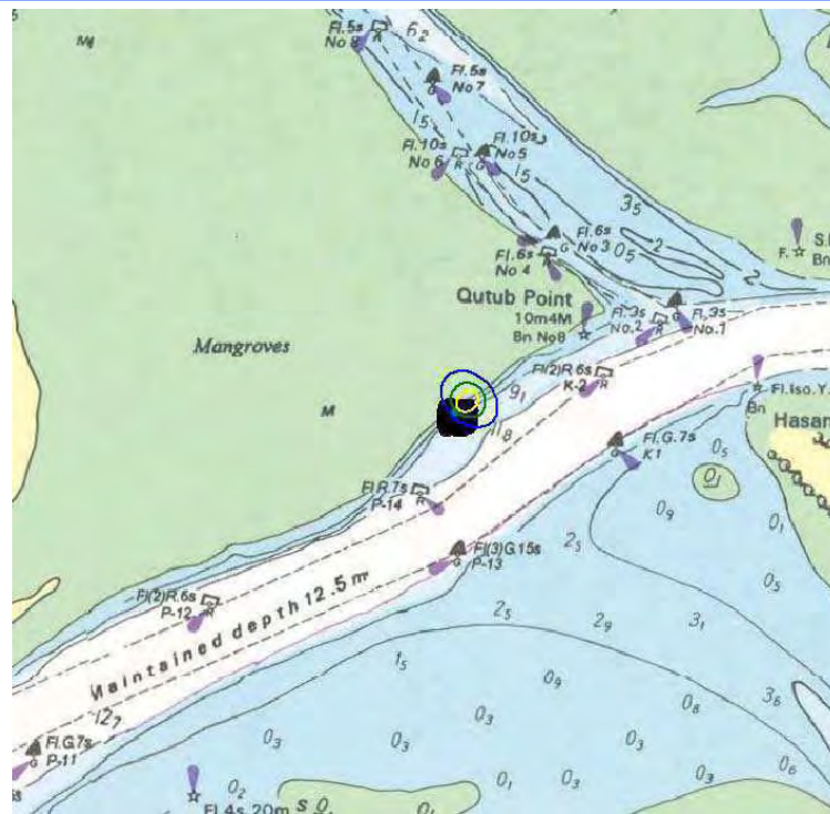
Figure 12 : Rupture of gas pipe on jetty, with failure of ESD. Jet fire radiation ellipse SW Monsoon / Day-time conditions, wind from SW Blue: 4 kW/m 2 ; Green: 12.5 kW/m 2 ; Yellow: 37.5 kW/m 2
