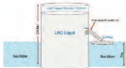
Figure 1: LNG Outflow from a Hole above the Water Line
