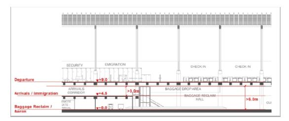
Figure 3-7 Layout of proposed building levels
