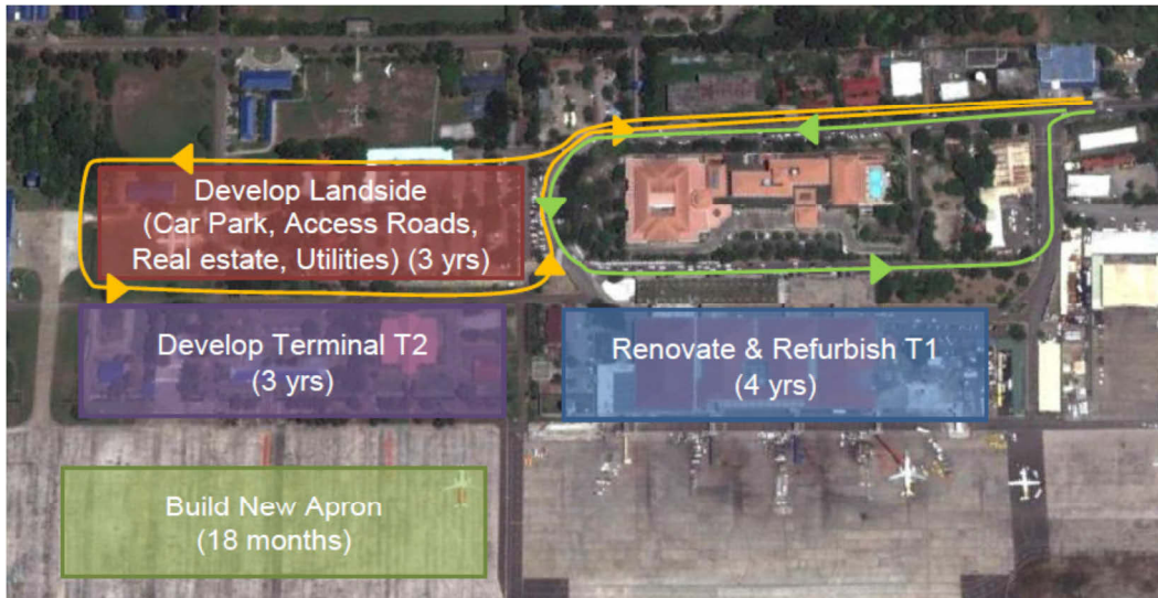
Figure 3-1 Development plan and schedules for the new airport
