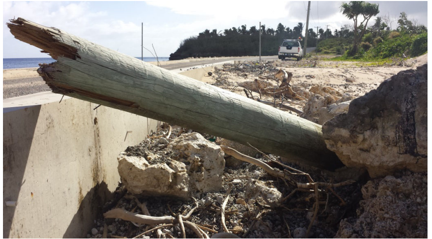
Photo 2: Poles snapped into pieces by cyclone.
