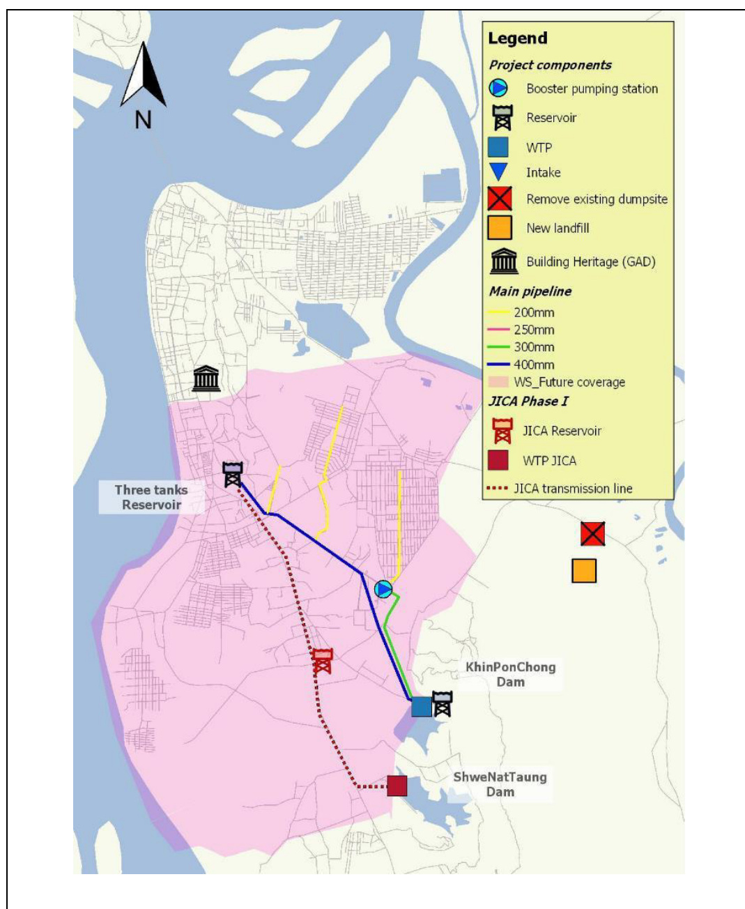
Figure 3-1: Proposed Third GMS Project Components in Mawlamyine
